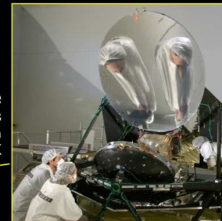
Planck Telescope 1.5x1.9m off-axis Gregorian T = 50 K
